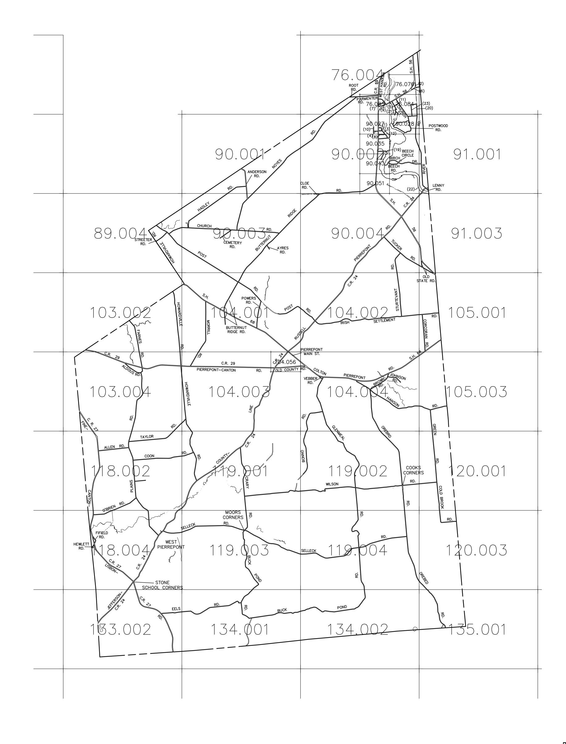
NOTE: A SERIES OF SQUARE OR RETANGULAR PARCELS (OF LESS THAN ONE ACRE) HAVING TWO OR FOUR EQUAL SIDES ARE USUALLY DIMENTIONED ON THE FIRST AND LAST LINE OF THE SERIES ONLY. ALL THE OTHER PARALLEL LINES IN THIS SERIES OF LOTS ARE TO BE CONSIDERED AS BEING THE SAME LENGTH.
